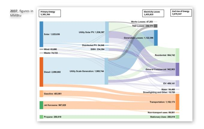
**Figure 3**: Energy Flow Diagram (2037)
