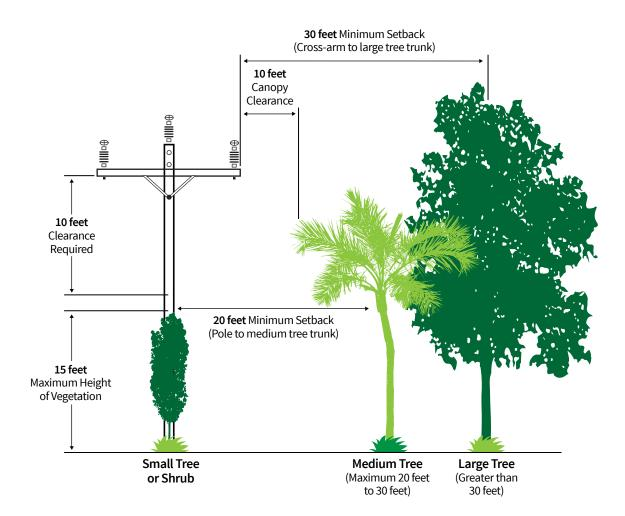
**Small trees** or **shrubs** planted near or underneath poles or power lines should maintain a clearance of 10 feet from the power lines (from the top of the tree).
