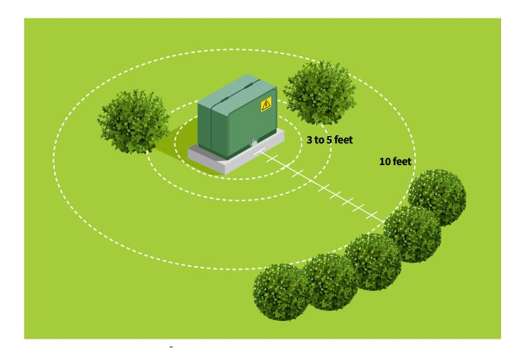
Stay well away from Padmount Transformers and Transformer Cabinets. They are green in colour. Areas around **Padmount Transformers** and **Transformer Cabinets** should be clear at all times to allow maintenance and repairs, especially in times of emergency.
