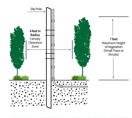
The **dip pole f**or an underground power line must be cleared at all times at a radius of **4 feet**.
