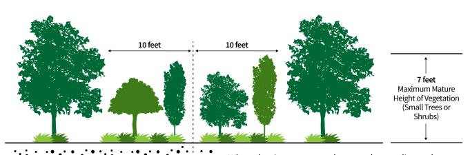
When planting near an underground power line, only trees with a mature height of **less than 7 feet** can be planted within **10 feet** of the centre of the underground power line.
